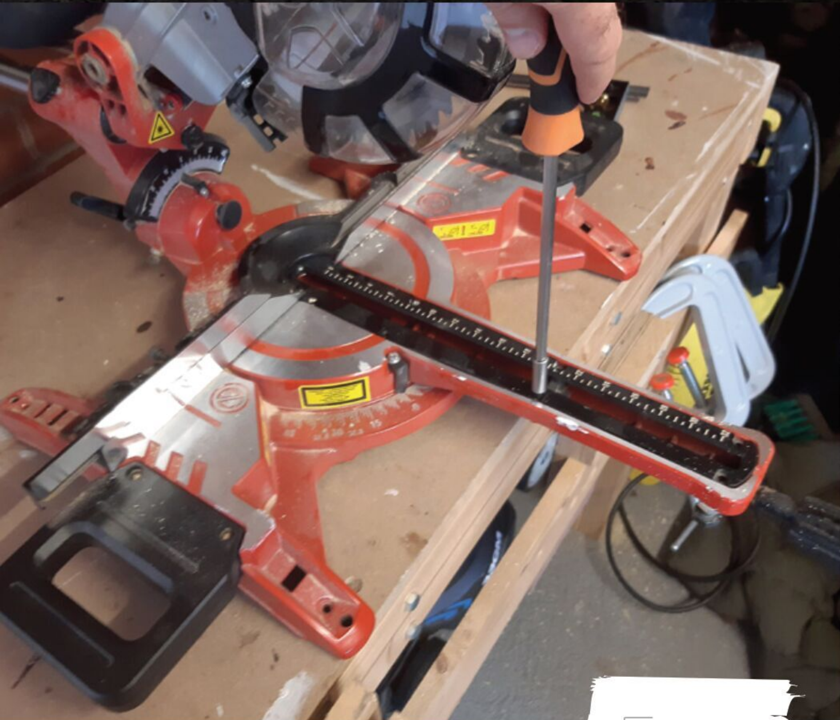
Above ♦ Just a few screws hold the clearance plate in place
