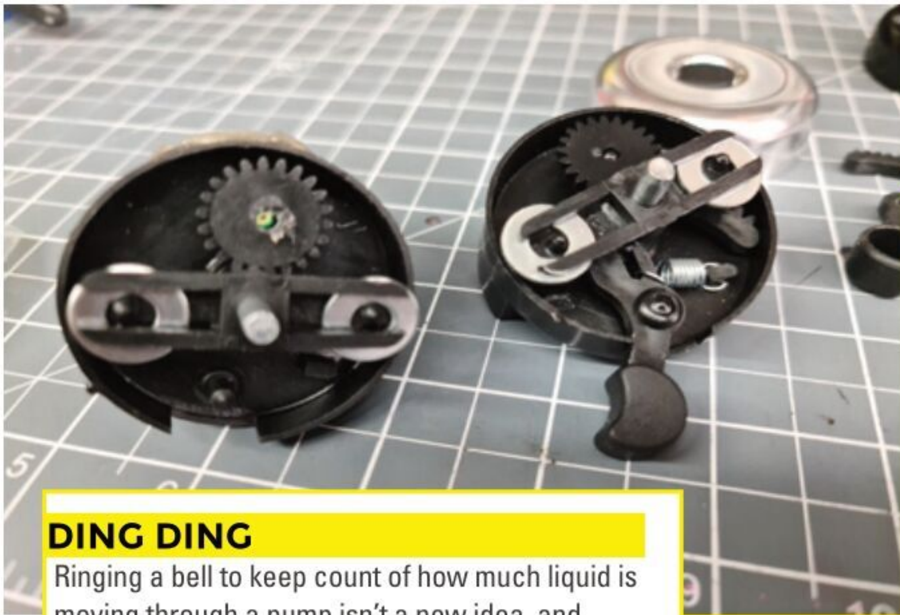
Left ← You can see that the interior of the bell is mechanically very simple, and modifying the bell to work with an electric motor needs nothing more than a drill and a hot glue gun. This photo shows the original bell, and the modified bell next to each other. The total cost of making an electric bell this way is around £5, and the sound is more distinctive than an off-the-shelf buzzer
